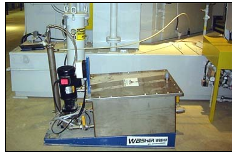
Washer Washer 1 with optional membrane housing, recycles alkaline cleaning solution
